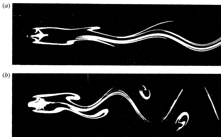
Figure 1. von Kármán vortex street, stretching and folding (cf. Bergé et al. 1984).
